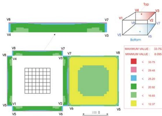
Figure 7. Charge Density Distribution over the Rectangular Volume Surfaces:  $\rho_1=200\Omega\cdot\text{m}$  and  $\rho_2=1000\Omega\cdot\text{m}$ . Volume Dimensions Are  $200\text{ms}\times 200\text{ms}\times 20\text{m}$ .
