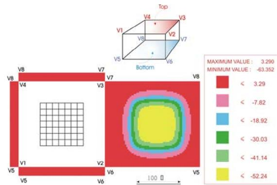
Figure 9. Charge Density Distribution over the Rectangular Volume Surfaces:  $\rho_1=1000\Omega\cdot\text{m}$  and  $\rho_2=200\Omega\cdot\text{m}$ . Volume Dimensions Are  $200\text{ms}\times 200\text{ms}\times 20\text{m}$ .
