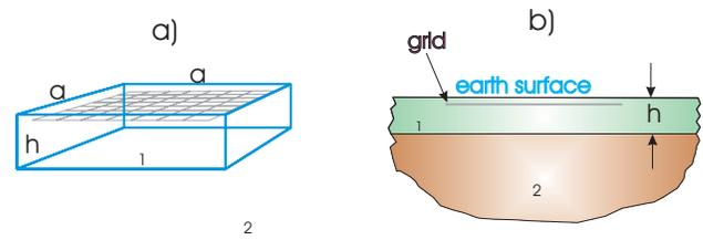
Figure 5. Rectangular (a) and Horizontal Two-Layer (b) Soil Models.
