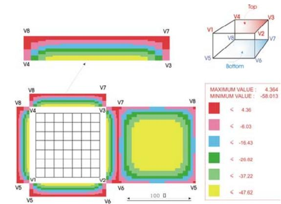
Figure 8. Charge Density Distribution over the Rectangular Volume Surfaces:  $\rho_1=1000\Omega\cdot\text{m}$  and  $\rho_2=200\Omega\cdot\text{m}$ . Volume Dimensions Are  $120\text{ms}\times 120\text{ms}\times 20\text{m}$ .
