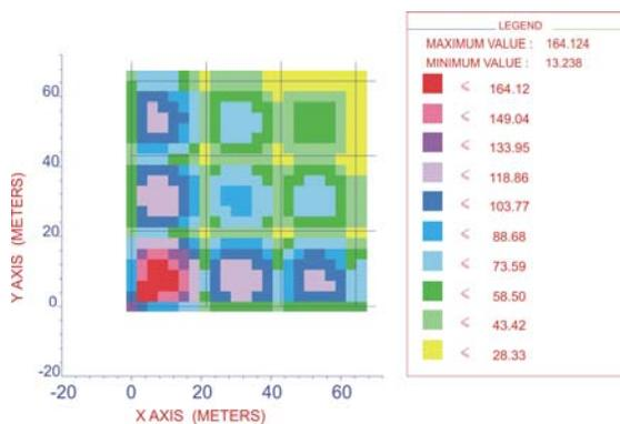
Figure 11. Touch Voltages over the Immersed Region of the Grid: Rectangular Soil Volume.
