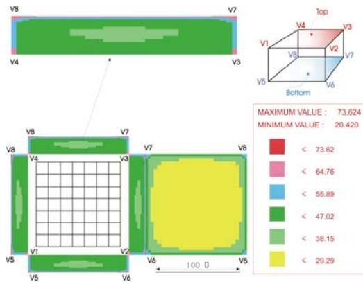
Figure 6. Charge Density Distribution over the Rectangular Volume Surfaces:  $\rho_1=200\Omega\cdot\text{m}$  and  $\rho_2=1000\Omega\cdot\text{m}$ . Volume Dimensions Are  $120\text{ms}\times 120\text{ms}\times 20\text{m}$ .
