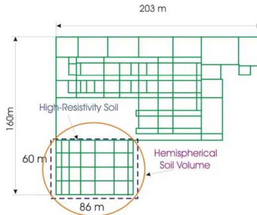
Figure 13. Grid Partially Immersed in High Resistivity Soil Volume.
