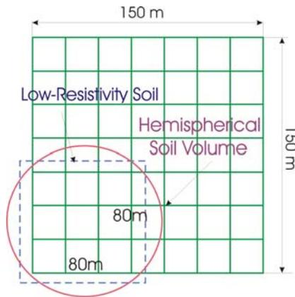
Figure 10. Grid Partially Immersed in Low Resistivity Soil Volume.
